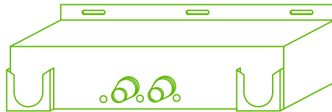
200 AMP TWO POINT JUNCTION UM6-20
